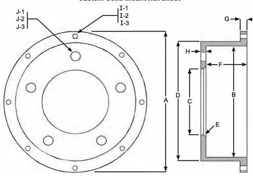
No Metric Sizes Please "A" (Outside Dia.) "B" (Inside Dia.)\_\_\_\_\_ "C" (Center Bore)\_\_\_\_\_ "D" (Face Diameter)\_\_\_\_\_\_ "E" (Chamfer size) "F" (Offset) "G" (Flange Thickness)\_\_\_\_ "H" (Face Thickness) "I-1" (No. Of Holes)\_\_\_\_\_ "I-2"(Bolt Circle) "I-3" (Size Of Holes)\_\_\_\_\_ "J-1" (No. Of Holes)\_\_\_\_\_ "J-2" (Bolt Circle)\_\_\_\_\_\_ "J-3" (Size Of Holes)\_\_\_\_ Material: Aluminum / Steel
